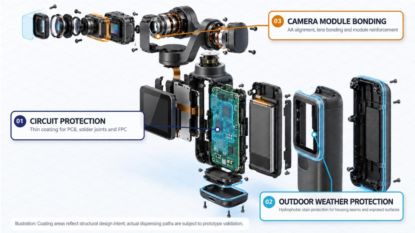
Figure 2 Pocket Gimbal Camera Exploded View and Material Application Areas
